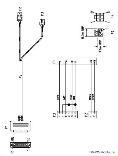
Figure 18 - Remote Mount Standard Accessory Cable 19B802554P6
